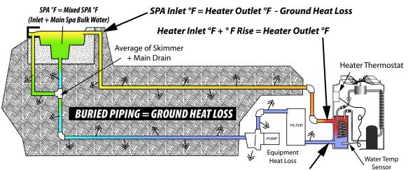
SPA Outlet °F - Ground & Equipment Heat Loss = Heater Inlet °F
